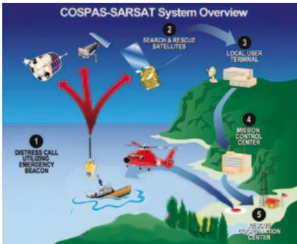
5km (3 miles). The coded message identifies the exact vessel to which the EPIRB is registered, or the person the PLB is registered to. This information allows the rescue services to eliminate false alerts and launch an appropriate rescue.
