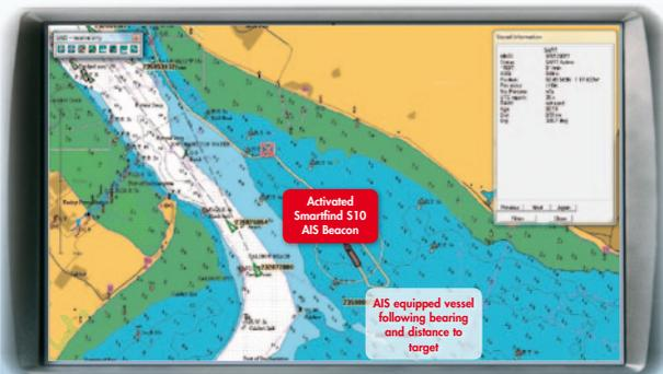
AIS equipment\* displays the icon (pictured above). Precise target survivor information becomes viewable when the chart plotter/ECDIS\* cursor is positioned over the alert icon.
